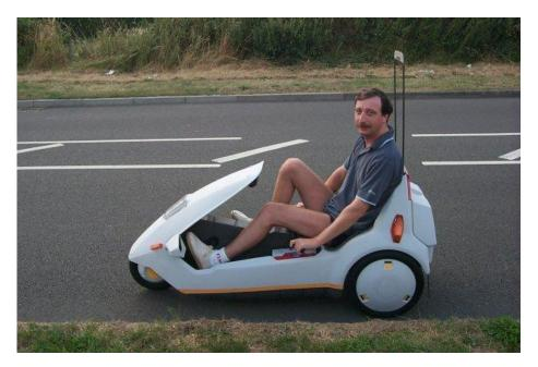
Technology developed in isolation doesn't often succeed –Sinclair C5 •One man's vision -IQ149 •Cost same as 2<sup>nd</sup> hand car •Designed for urban use (weighed 30KG) •Top speed 15mph (halved in cold weather)
